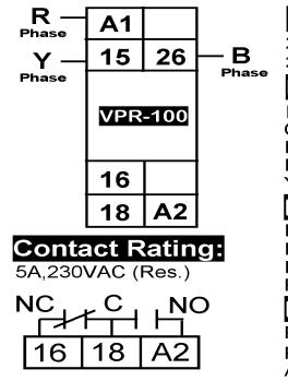
INPUT Voltage: 280 to 520VAC (L-L) 3-Phase - 3W LED Indications: **F-LED** UV/OV LED OFF: Healthy OFF: Healthy RED: PL RED: UV Blinking: PA Blinking: OV YELLOW: PS FUNCTION: Phase Loss<280VAC (L-L) Phase Asymmetry >=40V Fix Hysteresis: 6V Fix Rated Voltage: 415VAC (L-L) **Delay Time:** Power ON & Trip Delay: 5 Sec. PS,PL: <200ms Asymmetry: 5 Sec
